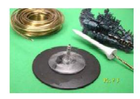
Apply super glue to threads and shaft of screw and screw the large end of the golf tee onto it to contact the topside of the small
